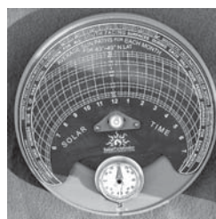
Solar Path Finder : Check shading of proposed PV site.
